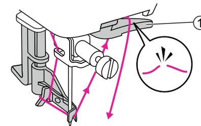
13. To cut the excess thread, take thread end and gently slip it over the thread cutter located on the right of the needle.
