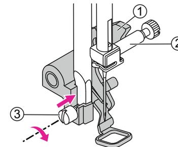
The embroidery foot lever will be against the top of the Needle clamp screw, then tighten the screw by using the screwdriver.
