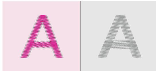
When the bobbin thread is visible on the front of the fabric, the thread tension is too tight for embroidering. To reduce the tension, press the "-" button.
