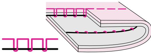
Thread tension is too loose for straight stitch sewing. To increase the tension, press the "+" button.
