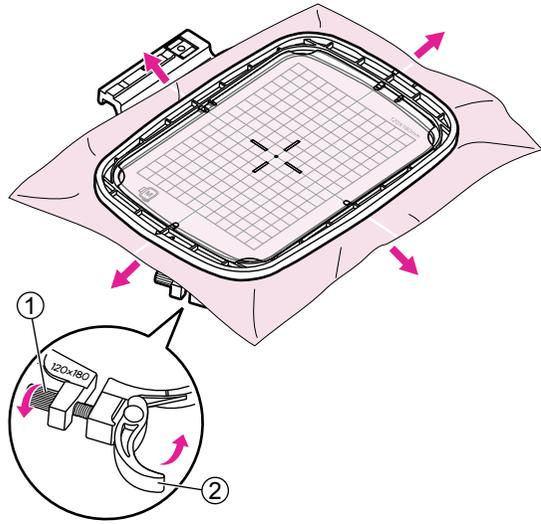
Place the inner hoop on the fabric and press firmly until they are securely fit to outer hoop perfectly. If the inner hoop cannot fit properly, loosen the outer hoop's fastening screw and adjust until fitted.
