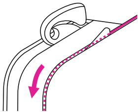
6. Continue to guide the thread into the silver discs to keep the thread in proper tension.
