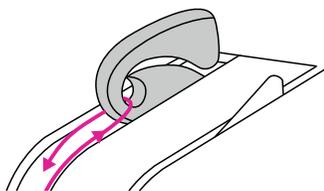
8. Pull the thread to the top then pass the thread through the slotted eye of the take-up lever. Guide the thread down afterwards.
