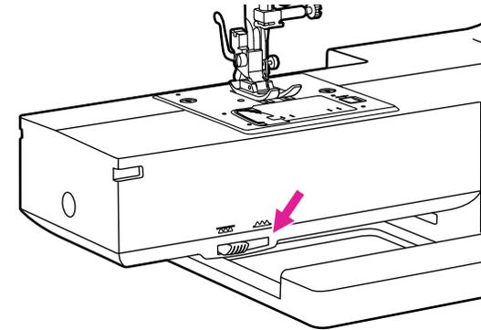
The drop feed lever can be seen on the base at the front side of the sewing machine.
