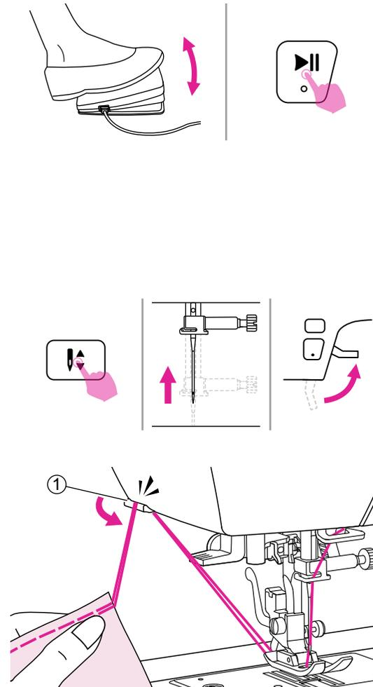
7. Slowly press down the foot control or press the start/stop button to start sewing. Release the foot control or press the start/stop button again to stop the machine.
