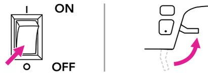
Turn the power switch to off ("O"). Raise the presser foot lifter.
