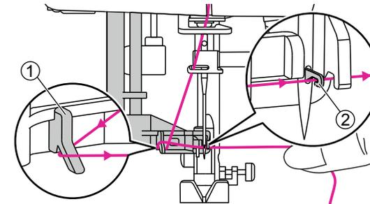
12. Pass the thread around the thread guide. Take the thread in front of the needle and make sure it is under the hook pin.
