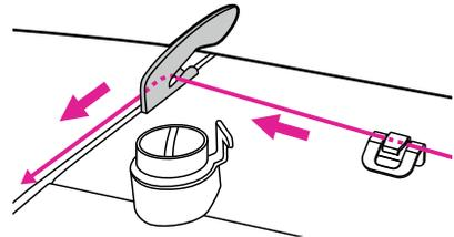
5. Guide the thread ahead and pull the thread through the pre-tension spring as illustrated.
