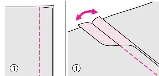
Working on the right side of the fabric, place the center of the presser foot on the seam line of the joined fabrics and stitch over the seam.
