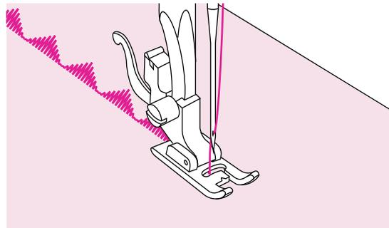
This foot has a groove on the underside which allows dense stitching to pass freely underneath.
