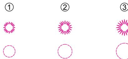
Press the "-" or "+" stitch width adjustment to button select the eyelet size.
