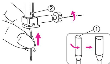
Inserting a 75/11 needle, keep the flat side of the shaft to the back.
