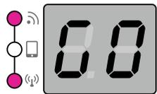
Start the App and the connection will follow automatically. When the connecting is done, the screen shows "GO" and the connection with the App is successful.
