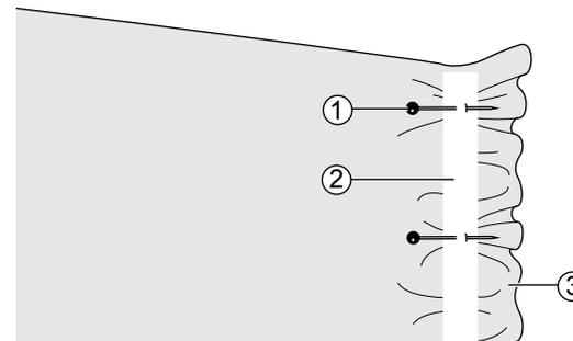
Pin the elastic tape to the wrong side of fabric at a few points to make sure that the tape is uniformly positioned on the fabric.
