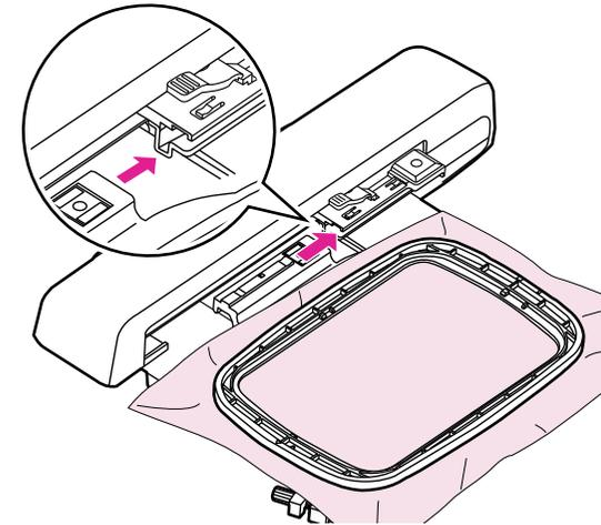
The embroidery hoop has two built-in sizes which are 120x80mm and 50x70mm, respectively. Select the corresponding size according to the image design.
