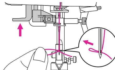
14. Raise the lever, the hook will rotate and pass the thread through the needle eye to form a loop.
