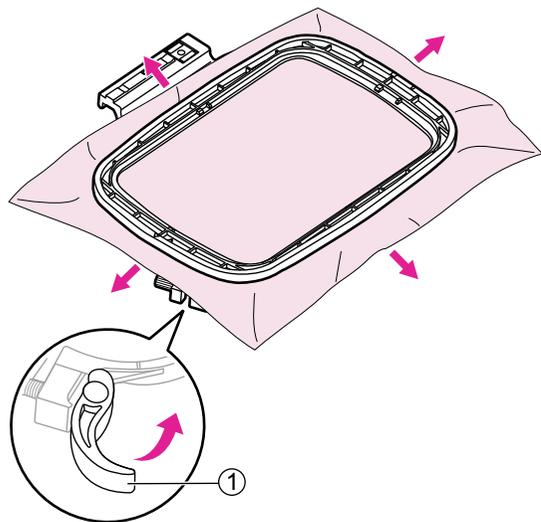
Place the inner hoop on the fabric and press firmly until they are securely fit to outer hoop perfectly, pull the fabric from the four sides marked with the arrows so that the fabric is stretched drum-tight in the hoop, and then press the inner hoop downwards so that it sinks into the outer hoop a little and close the quick release device.
