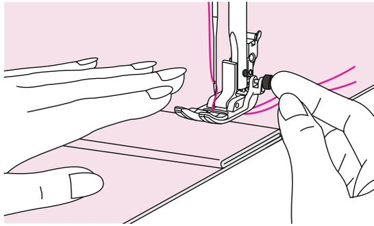
When you reach the point of an increased thickness, lower the needle and raise the presser foot. Press the toe of the foot to the horizontal line and push in the black button, then lower the foot and continue sewing.
