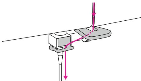
9. Pass the thread behind the flat, horizontal thread guide. Use the needle threader to thread the needle.
