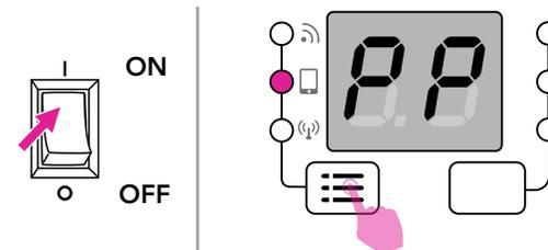
Turn on the power, and check if the screen shows "PP" and the second light is on. If it is not, please long press the connection mode switch button to switch the light.
