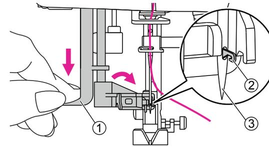
11. Pull down the lever to the very bottom. When heard a "click" sound, it will be on the right position to do the needle threading and the hook pin passes through the needle eye.
