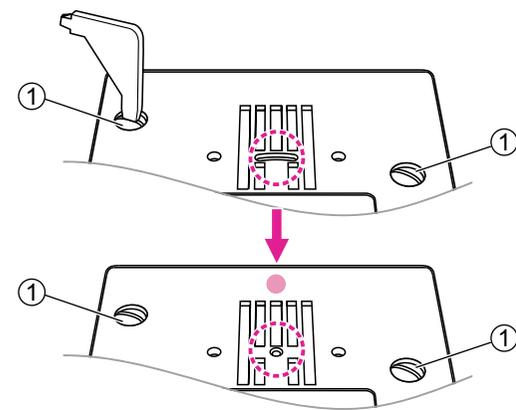
Remove the screws on the needle plate then remove the needle plate.
