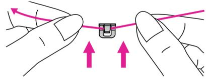
4. Draw the thread from the spool and place the thread in between the upper thread guide.
