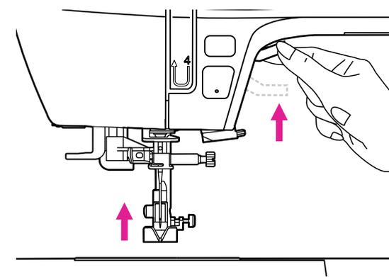
When sewing multi-layers or thick fabrics, the presser foot can be further raised up manually to allow enough space for your sewing work.
