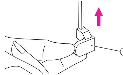
Raise the presser foot and cut the thread. To sew over the same buttonhole, raise the presser foot (it will return to its original position).
