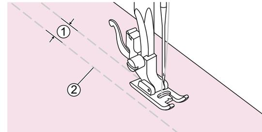
Increase the stitch length to maximum, set the tension below 2 and basting lines 1cm across the area to be smocked.
