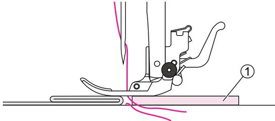
You also can place another piece of fabric with the same thickness at the back of the seam. Or support the presser foot while feeding by hand and sewing toward the folded side.
