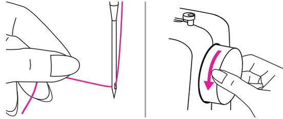
Hold the upper thread with your left hand. Turn the handwheel towards you (counter-clockwise) to lower the needle down below the needle plate then raise it to bring the bobbin thread up.
