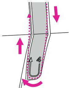
7. Pass the thread under the take-up spring then pull it upwards as arrow marks illustrated.
