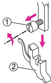
Loosen the screw counter-clockwise to remove the presser foot holder.
