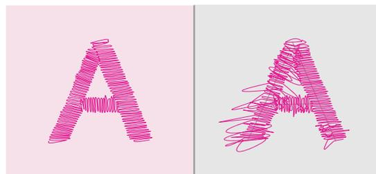
When the upper thread has slack, the thread tension is too loose for embroidering. To increase the tension, press the "+" button.
