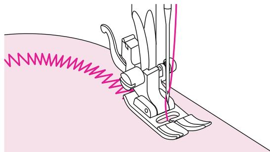
When sewing along a curve while using a zigzag stitch, select a shorter stitch length in order to obtain a finer stitch.
