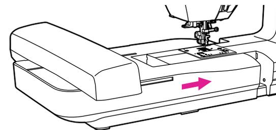
Slide the embroidery unit onto the machine arm. Push lightly until the unit clicks into place.
