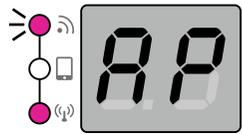
When the screen shows AP and the WiFi light start flashing, the machine is ready to connect with the App.
