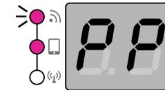
The WiFi light will start flashing, which means ready to connect machine.
